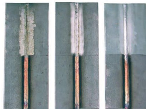
GRINDING POLISHING PICKLING INCREASING CORROSION RESISTANCE →
